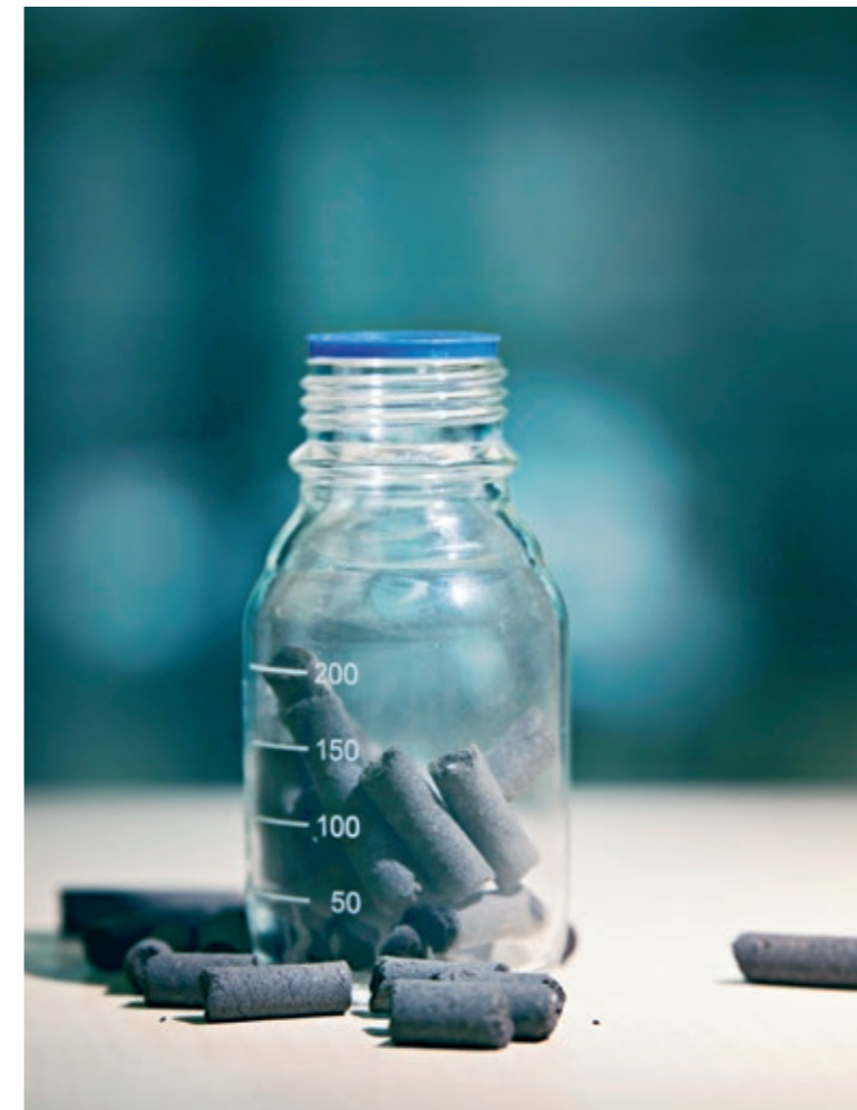
The economic prospects for Eawag's dried faecal sludge pellets, which can be burned, are excellent, including for the southern hemisphere (see p. 32 f.).
