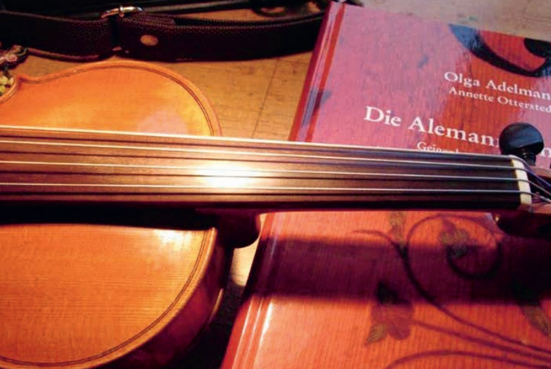
Hard to distinguish from the original: A violin with a fingerboard made from "Swiss Ebony" instead of genuine ebony. (Photo: Wilhelm Geigenbau AG, Suhr)
