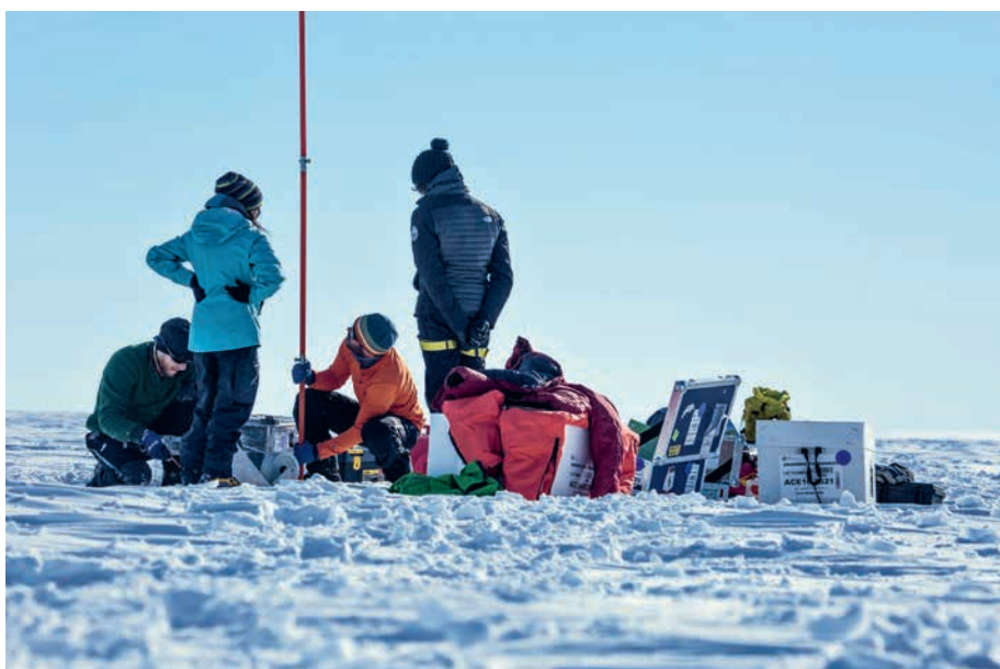
Core drilling on the Mertz Glacier as part of the SubICE project. The project, which was led by Liz Thomas, has set out to "read" the climate of the Antarctic from different ice samples. (Photo: Noé Sardet/Parafilms/EPFL)
