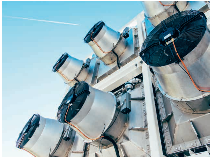
The ETH spin-off Climeworks, which was founded in 2009, put its first commercial plant into operation in Hinwil, filtering carbon dioxide (CO 2 ) from the air. (Photo: Julia Dunlop/Climeworks)
