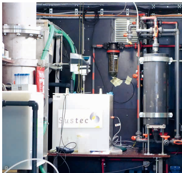
Energy harnessed from sludge through fermentation into biogas thanks to "Horizon 2020". (Photo: Eawag)
