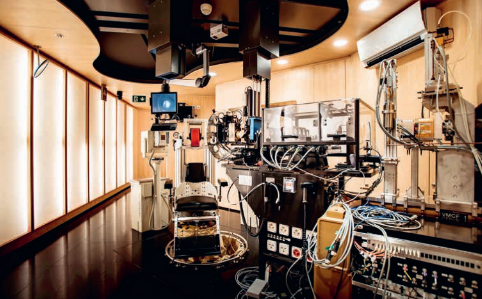
OPTIS2, the therapy facility for the treatment of ocular tumours, is based on the OPTIS irradiation system. (Photo: Mahir Dzambegovic/PSI)
